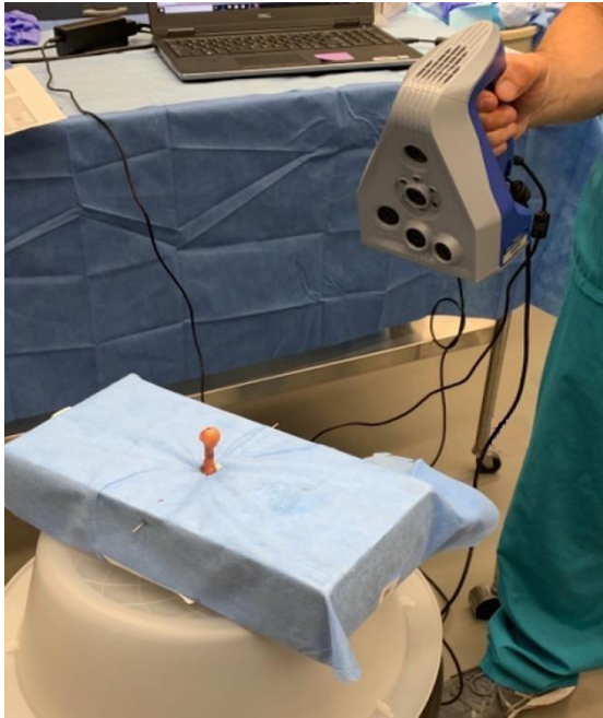
Figure 4. The Artec Space Spider 3D surface scanner was used to digitize the metacarpal head
